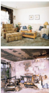
Photos of the same living room after fires with a sprinkler (top) and without a sprinkler (bottom).
